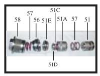
2. Remove valve adapter (56) and tension spring (57) with pull-out tool size 5. There is an O-ring (51G) under both the suction and the discharge valve each of which can be removed with a bent piece of wire. To disassemble unscrew the spring tension cap (51A) and press the valve seat (A) out of the spacer pipe (E). Check sealing surfaces and replace worn parts. Check O-rings and support rings. Reinstall all parts in reverse order and tighten plugs (58) to 107 ft. lbs.
